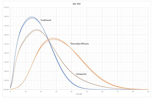
Figure 4 - BEL PDF at 6.0 GHz, 6.5 GHz and 7.0 GHz (0 degree elevation angle)
