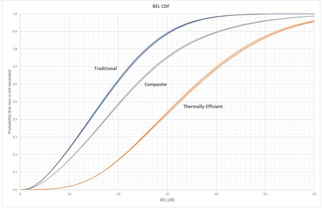
Figure 3 - BEL CDF at 6.0 GHz, 6.5 GHz and 7.0 GHz (0 degree elevation angle)
