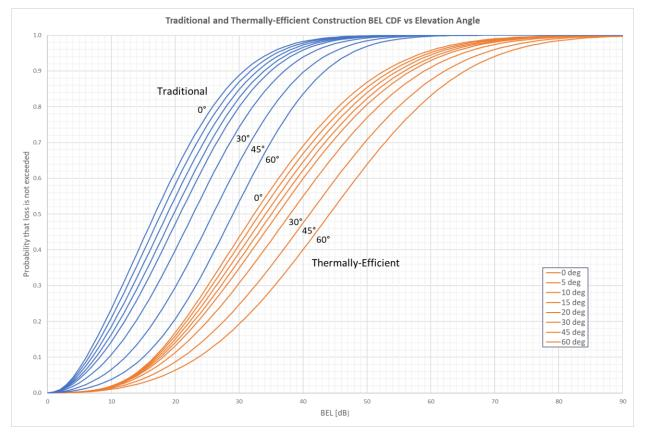
Figure 5 - BEL CDF at various elevation angles (6.5 GHz)
