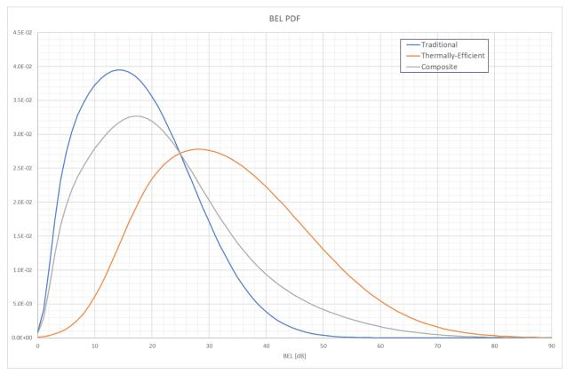
Figure 2 – PDF Frequency 6.5 GHz Elevation Angle 0 degrees 70/30 Composite
